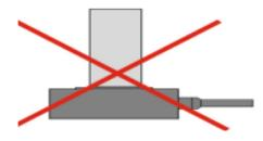
It is forbidden to mount the load on one side of the moving platform, which will cause serious damage to the product, as shown in the figure below.
