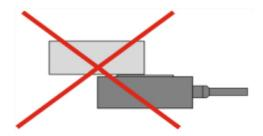
Excessive length of screws selected in the fastening and connecting process will lead to failure in installation or leakage of bolts, which will expose the product and scratch the product, affecting the motion accuracy of the product. Short bolts will lead to insufficient compactness of the connection and easy looseness, which will damage the internal structure of the product during operation.
